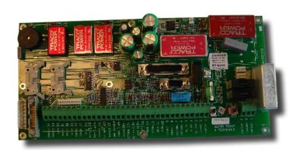
The PT-G041 is a PCB Terminal Board, Colour screen version, for the SKIPPER GDS101 Navigational Echo Sounder.
